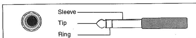
b) JACK INPUTS Unbalanced Signals
