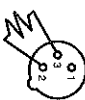
Termination reduces signal errors and avoids signal transmission problems and interference. It is always advisable to connect a DMX terminal. (Resistance 120 Ohm 1/4 W) between PIN 2 (DMX-) and PIN 3 (DMX+) of the last fixture.
